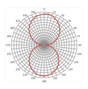
Angular Sensitivity (Relative Read Range vs. Orientation)
