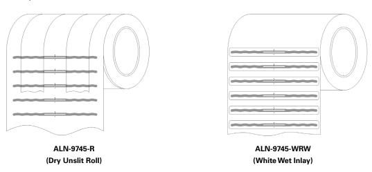
Standard Alien Inlay rolls unwind with metal antenna side facing outward, with respect to the core.
